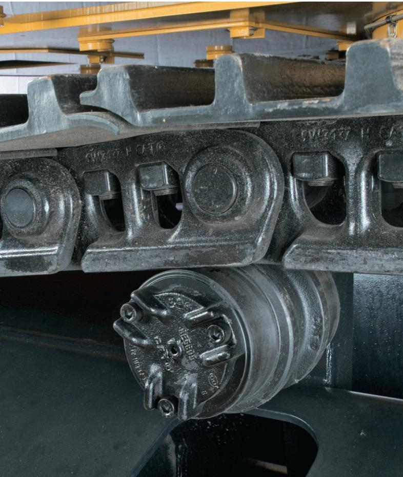
Caterpillar uses advanced engineering and software to analyze all structures, creating a durable, reliable machine for the toughest applications. More than 70 percent of the structural welds are robotic and achieve over three times the penetration of manual welds. These structural components and the undercarriage are the backbone of the machine's durability.
