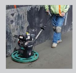
Allows finishing within 7/16" of any obstruction
