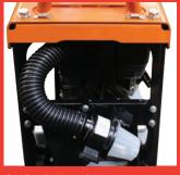
**Cyclonic pre-cleaner** - significantly reduces maintenance frequency and prolongs maximum efficiency of engine.
